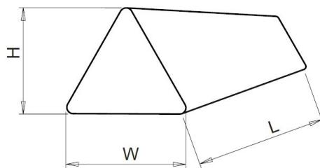
Extruded fibre concrete spacer with triangular section
